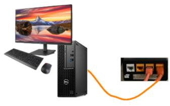
Now that the norm is to use a laptop to enable remote work, it is more common for that ethernet cable to connect the data jack in the wall to a docking station on the desk. When you connect the laptop to the docking station, the wired connection is extended to the laptop.
